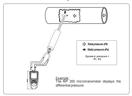
With the dynamic pressure in mm CE or in Pa, we can calculate the air velocity in m/s, with the simplified BERNOULLI formula:
